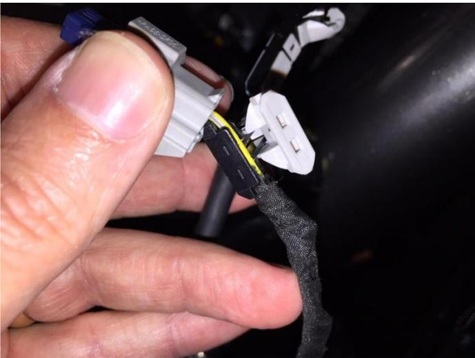
The scotch locks should look flat when installed correctly. Scotch locks are removable if the factory BOV is to be re-installed. Secure plug by using the supplied cable ties.
