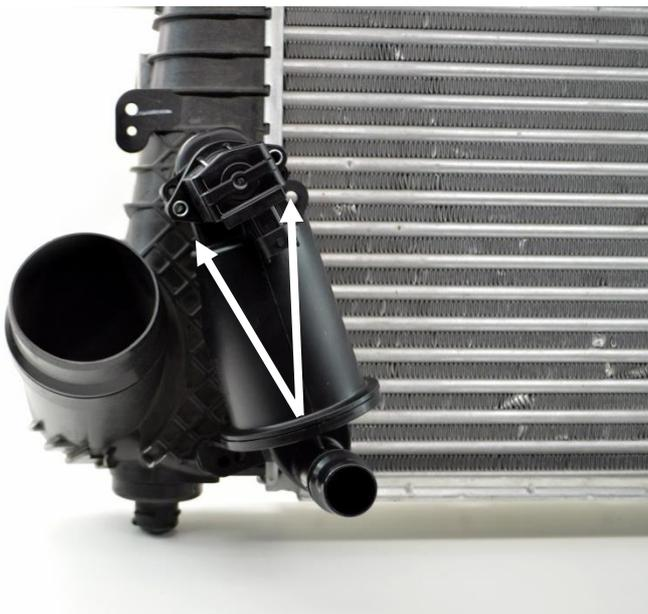
Remove the BOV chamber by turning it upwards. The BOV chamber should just unscrew.
