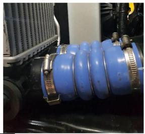
Removing BOV Chamber from Plumb back Hose
