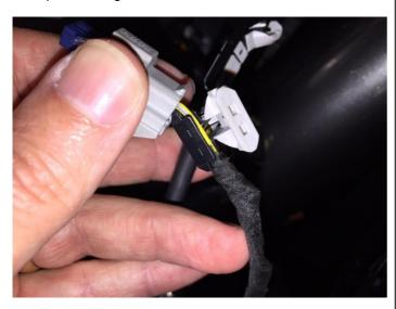
The scotch locks should look flat when installed correctly. Scotch locks are removable if the factory BOV is to be re-installed. Secure plug by using the supplied cable ties.
