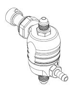
Patent pending Pro OPR is an oil pressure regulation system for turbochargers. It helps prevent compressor or turbine stage oil leaking/smoking and takes the guesswork out of oil restrictor sizing for more efficient and effective oil delivery. The Pro OPR increases the Oil Pressure relative to the reference boost pressure. A true plug and play setup for oil feed to turbochargers, additional restrictors not required.
